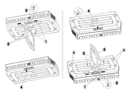
**NOTE:** Use caution to avoid damaging the LCD screen and the main unit when converting this unit from an under-counter unit to a countertop unit. Leave the protective plastic on the screen until this procedure is completed.
